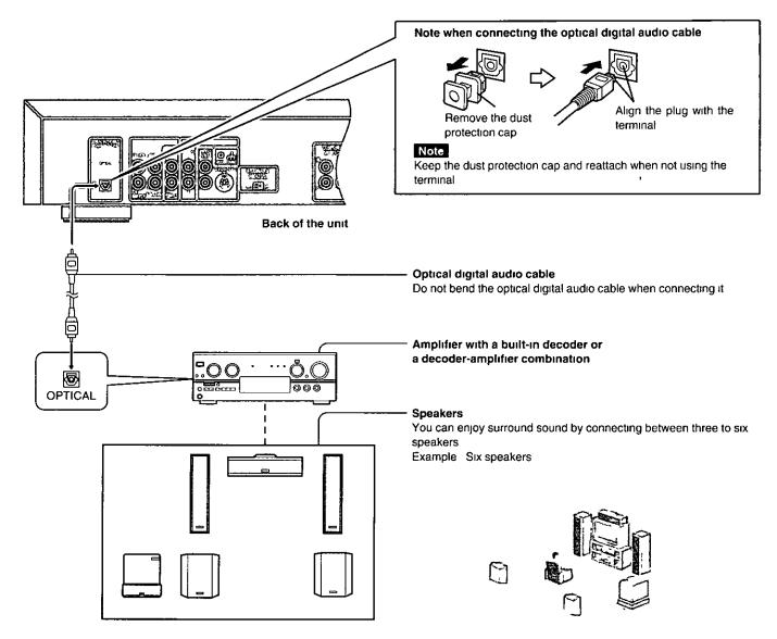
2 Adjust the setting to suit the equipment you have connected (→ page 38 "Selecting digital output").
